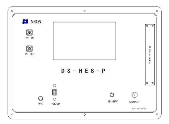
RF connector: SMA-K (Customized) DC connector: DE-9PS (Customized)
